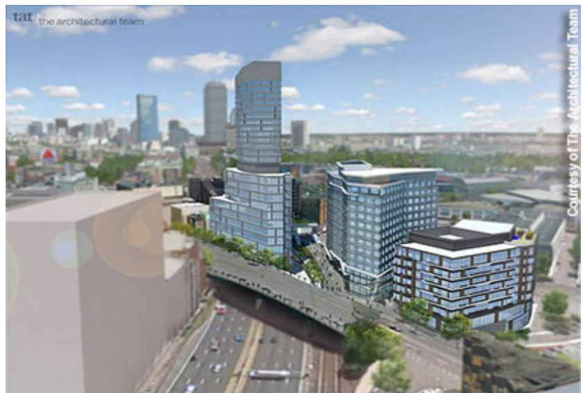
A $500-million air-rights project will place four buildings alongside of, and on top of, a decked-over stretch of the Massachusetts Turnpike.
